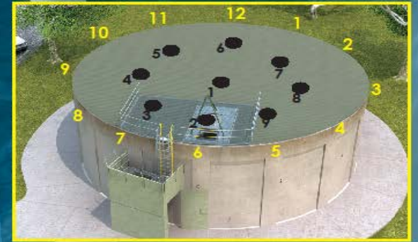
THE CENTRE POST IS #1 AND FURTHER NUMBERS RADIATE OUTWARDS IN A CLOCKWISE DIRECTION WITH #2 BEING NEAREST TO THE 6 O'CLOCK POSITION.
