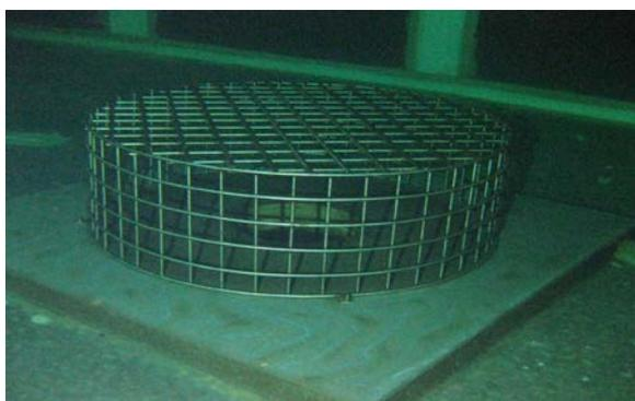
Figure 9 Outlet area cannot be cleaned
