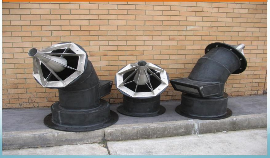
Outlet safety screens made from HDPE prevent sediment accumulation from entering the pipe work – they should fit the penetration closely to avoid internal sediment entrapment which is difficult to remove during normal cleaning operations.
