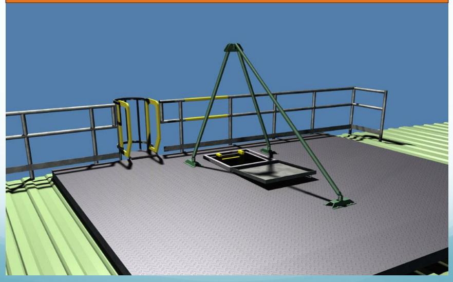
This new platform layout is a big improvement – it has a good slope for effective drainage and a rescue system is in place.
